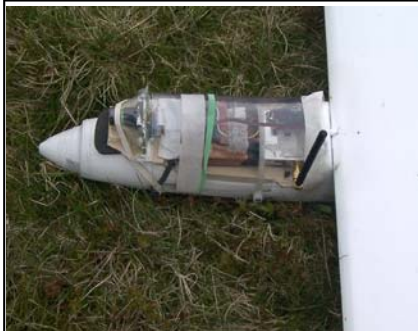
The camera & microwave Tx in the Diamond
