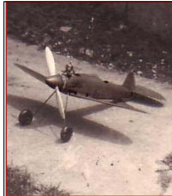
Phantom control line model popular in the 50's ~ usually powered by 1.5 cc diesel on 35ft lines ~ could get up a fair head of steam for those days
